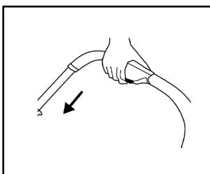
4. Press the safety catches (a) on both sides of the handle while pulling the secondary lock
