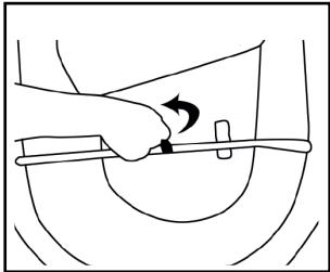
3. Press the buttons on the inside of the canopy to lower it. Pull to unfold the canopy again.
