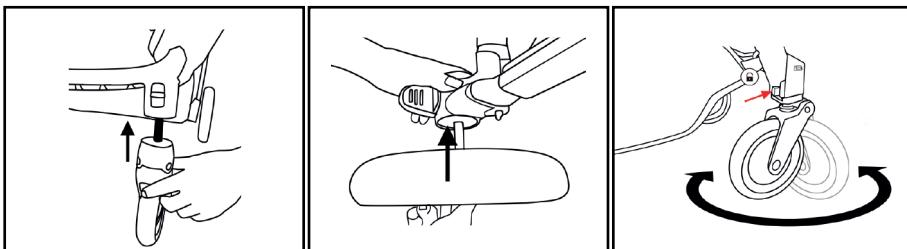
The stroller is equipped with front wheels that can either rotate freely or lock. It is suggested to use the fixed wheels on particularly uneven terrain. The wheels in swivel mode instead, can be used to improve the stroller's handling on regular road surfaces. To lock the wheel (against rotation), press the lock located at the top of each wheel (c).
