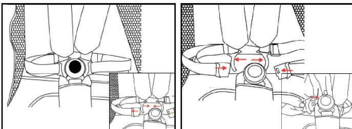
To unbuckle the lap strap, press the center buckle button to release all parts of the belt.
