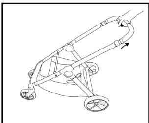
**4. Put the carrycot or the seat on the frame. Then press the adjust plastic and seat second lock to open the seat. The seat can be used in the direction of travel as well as in the opposite direction.**
