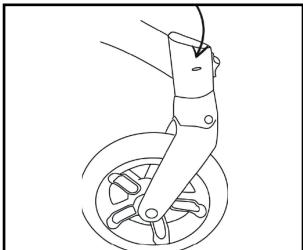
To release the rear wheel, press the button on the inside of the wheel.
