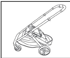
3. Press the telescopic handle button and pull the handle as low as possible.
