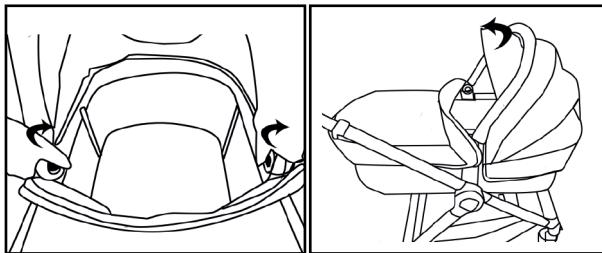
4. To fold the carrycot, loosen the metal reinforcements on the inside of the carrycot.
