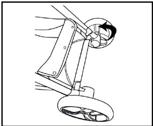
To disengage the parking brake push the pedal upward
